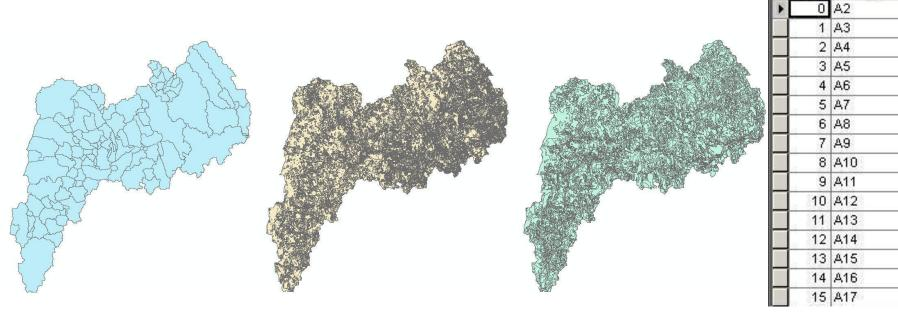
Basin Shapefile (Obtained from USGS StreamStats) Land Use Shapefile (Obtained from USGS Seamless) Soil Shapefile (Obtained from NRCS Soil Data Mart) Lookup Table (May be Customized By User)
