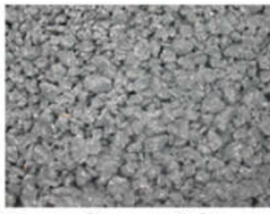
Porous Concrete (PC)
